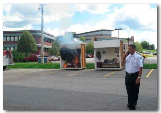
Photo 13: For training purposes, the fire sprinkler in the room was opened manually. Chief Caravasos explains to the RAs how effectively and quickly fire sprinklers control a room fire. After only a few seconds of sprinkler operation, the fire is knocked down.
