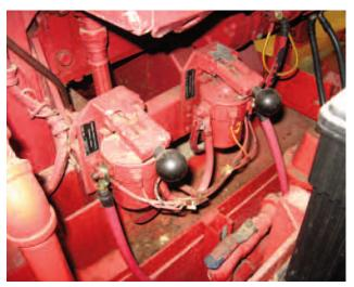
Photo 11: Battery contactor levers located on the side of a diesel engine.
